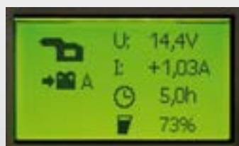
The current battery data: voltage, current, remaining operating time, capacity
