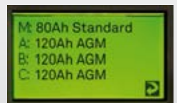
Display of the status of all batteries connected
