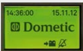
Start display: enter the menus by turning the button
